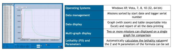
**TS Manager** – Validation software compatible with FDA 21 CFR Part 11 regulation, for SterilDisk (all versions), PasteurDisk Can, SterilDisk Can, S-Disk J ((all versions), P-Micro ((all versions), S-Micro ((all versions), P-Radio ((all versions), S-Radio (all versions), S-MicroW (all versions), L-Disk, supports DiskInterface HS Mini and DiskInterface HS.
