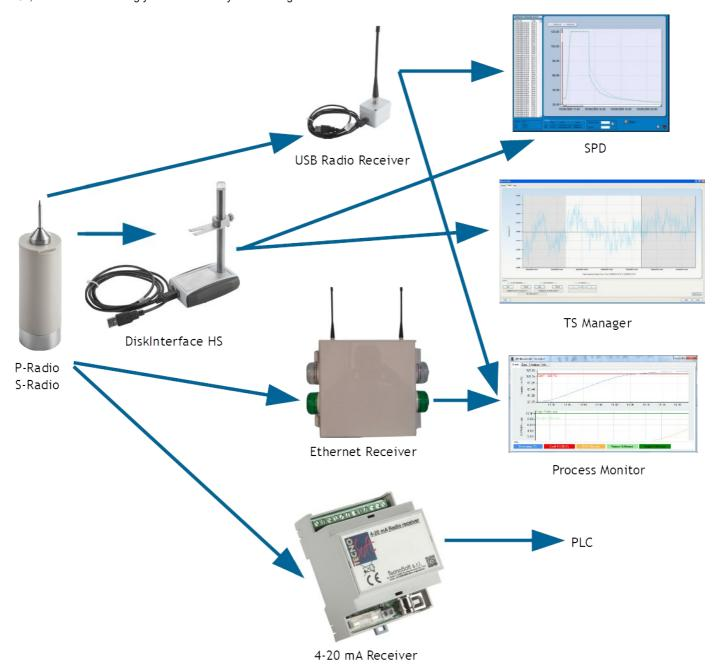
SPD – SterilDisk, PasteurDisk Can, SterilDisk Can, S-Disk J, P-Micro (all versions), S-Micro (all versions), P-Radio, S-Radio, S-MicroW (all versions), L-Disk management software, supports DiskInterface HS Mini, DiskInterface HS and USB Radio Receiver. Downloadable from Tecnosoft website and included with the interfaces.
