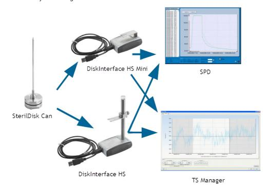
**SPD** – SterilDisk, PasteurDisk Can, SterilDisk Can, S-Disk J, P-Micro (all versions), S-Micro (all versions), P-Radio, S-Radio, S-MicroW (all versions), L-Disk management software, supports DiskInterface HS Mini, DiskInterface HS and USB Radio Receiver. Downloadable from Tecnosoft website and included with the interfaces.
