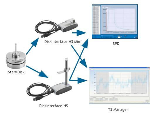
SPD – SterilDisk, PasteurDisk Can, SterilDisk Can, S-Disk J, P-Micro (all versions), S-Micro (all versions), P-Radio, S-Radio, S-MicroW (all versions), L-Disk management software, supports DiskInterface HS Mini, DiskInterface HS and USB Radio Receiver. Downloadable from Tecnosoft website and included with the interfaces.
