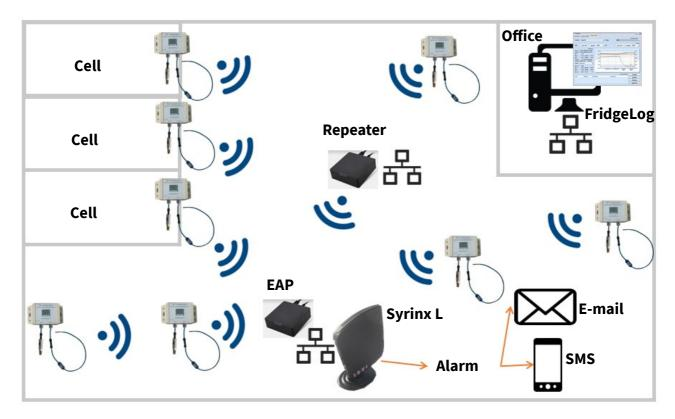
ZED IT - Radio module without intelligent sensors, can accept up to two intelligent sensors among the ones available, in any combination. Has 1 button for ON/OFF and diagnosis. Upon purchase you can add external power and/or display+keyboard modifications. Can be configured (number and type of sensors, radio channel, radio network, repeater function) via USB. See further for available sensors.
